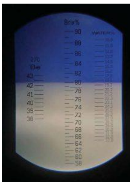
Figure 4: Honey Refractometer eye piece readings/results (Source: Bäckmo, H. (2023, September 13))
