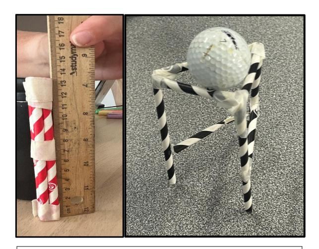
The **image on the left** is a failed project: The tower is built with 8 x 13cm vertical straws taped together, but there are no supports to stop it from bending or collapsing sideways.
