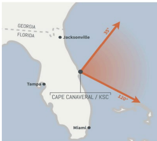
Figure 2. Roberts, T. (2019, March). Figure 3: Azimuth Limitations at Cape Canaveral and Vandenberg. [Map]. Centre for Strategic and International Studies. Retrieved April 16, 2023 from https://aerospace.csis.org/spaceports-of-the-world/
