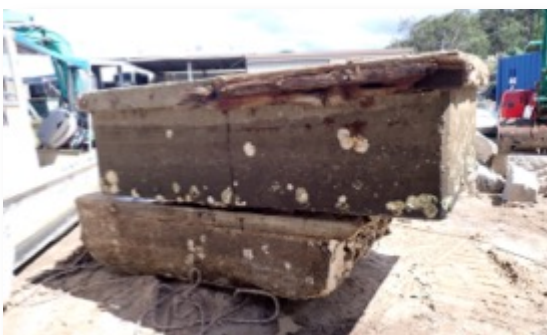
Timber logs from the bushfires washed into the Hawkesbury by floodwaters and concrete covered polystyrene pontoons decaying in the water
